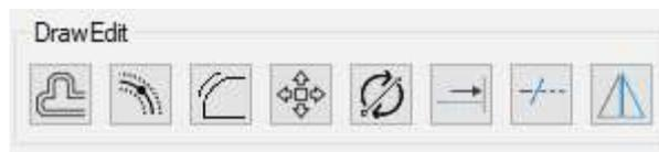
DrawEdit contains all the buttons that are used to make changes to the selected elements such as moving them, reversing the direction, making the fillet etc ...
